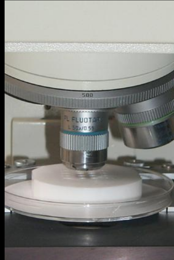
Upright microscope in reflection mode (no fluorescence)
