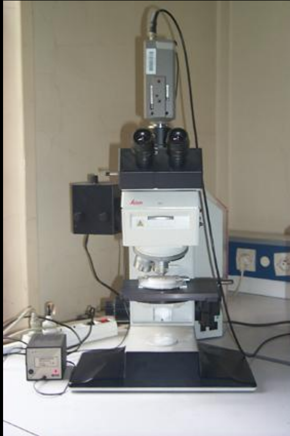
Upright microscope in reflection mode (no fluorescence)
