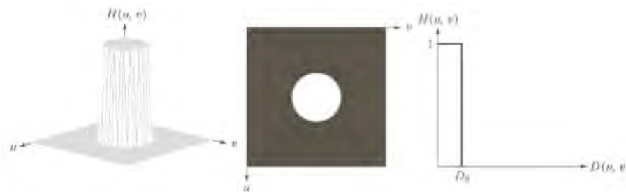
FIGURE 4.40 (a) Perspective plot of an ideal lowpass-filter transfer function, (b) Filter displayed as an image, (c) Filter radial cross section.
