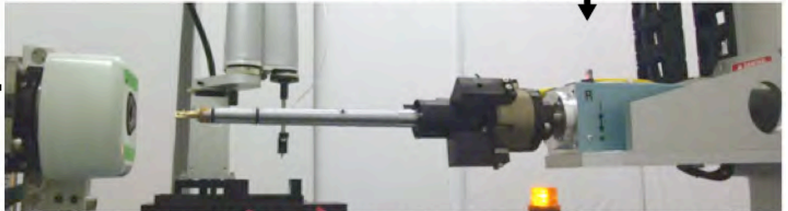
Robotic grid handling and automated image acquisition by EM
