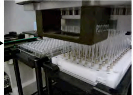
Automated grid staining on magnetic tray
